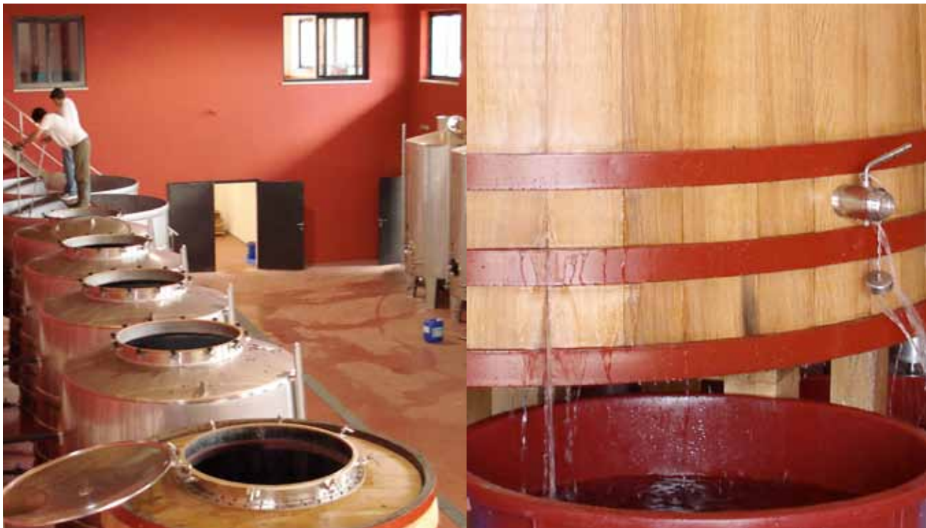
The heavy physical work of pigeage (punching down) atop stainless-steel tanks; the leaky reconditioned wooden vat, supposed to hold up to 4,000 liters of wine
